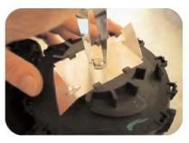
Lever the cutter and its support thanks to 2 screw drivers.
