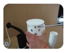
With the flat screwdriver unclip the basket from the motor cover's hooks.
