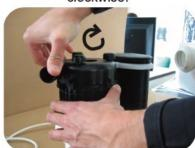
Verify that the small hole of the pressure chamber is not blocked.
