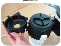
By maintaining the cutter (BEWARE!) unscrew the impeller anti-clockwise. Take out the washer.
