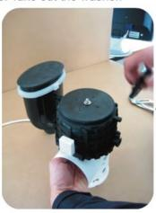
Verify that nothing is jammed in the axis in the impeller.
