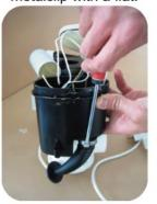
Insert the electric equipment back ( beware not to squeeze the cables ).
