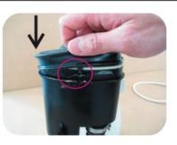
Position the 2 half-clips BETWEEN the membrane and the pressure chamber.
