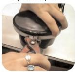
Press the membrane to check the free movement and correct switch clicking/activation.
