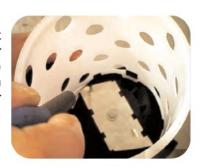
Thanks to a flat pinch, unclip the circlip of the cutter.
