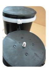
Screw back the impeller with washer and remount the pump body ( respect the mistake-proofing).
